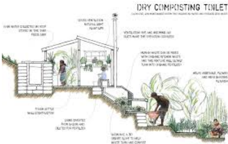
Figure: Dry composting toilet.
